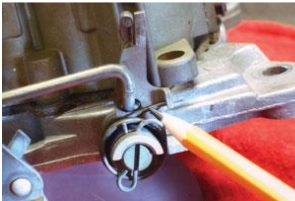
Photo 6: Metering rod travel can be easily checked by inserting an applicable tool into the front float bowl vent.
