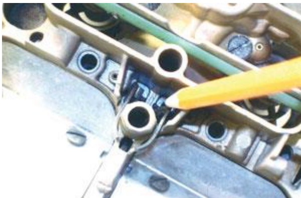
Photo 7: The secondary metering rod height adjustment should be checked to ensure delivering a correct secondary air/fuel ratio.
