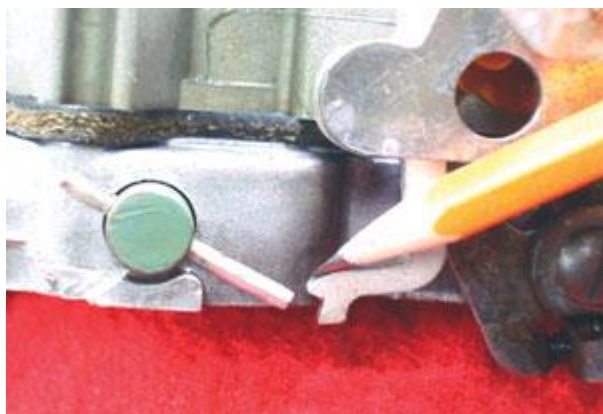
Photo 9: Make sure the secondary throttle lockout disengages when the choke valve opens.
