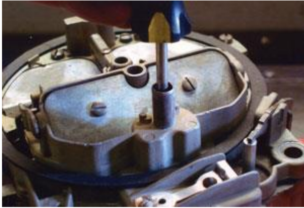
Photo 5: Metering rod travel can be easily checked by inserting an applicable tool into the front float bowl vent.
