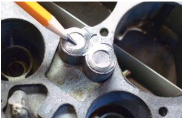
Photo 1: Leakage from the secondary metering well plugs are the most common Quadrajets failure.
